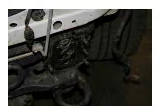
Center support bracket with has an extending mount coming off of it; this must be cut off in order for the bumper and/or winch to fit.
