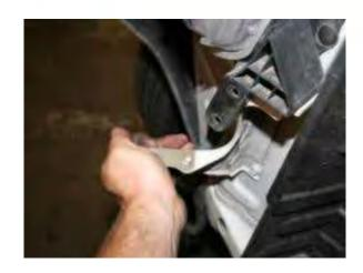
Locate the internal mounting brackets (pictured to the right). Install utilizing the oem flange nuts, it is recommended you install just the nuts on the inside of the frame initially.
