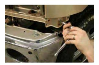
Now unbolt the chrome outer shell of the bumper to expose the aluminum bumper underneath.
