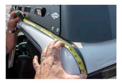
Our measurements indicated at 97/8)" mark for where to cut towards the rear. Place the mount bracket at this location and mark out your other edge for good cutting fitment.
