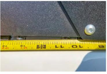
Once you have your dimensions with the tape measure shown above and verified by placing the mount bracket on the roof, mark with a sharpie where you'll need to cut the rubber trim.
