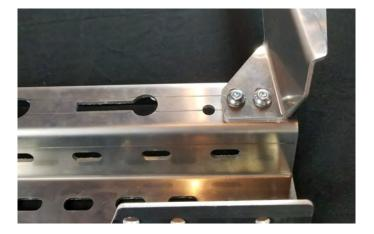
Lay out side fascia pieces and attach with 1/4" bolts (remember to hand tighten but keep loose).
