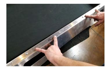
Next attach rear corner connectors with 5/16" bolts shown in photo below. (remember to hand tighten but keep fairly loose!)
