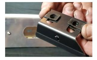
Once you've drilled out your roof holes around the vehicle and installed the riv nuts, place your mounting feet into position and tighten down into place with provided washers/bolts.
