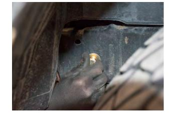
Attach provided clip piece onto the large frame bracket as shown in photo. These will be used to attach the included skid plate.
