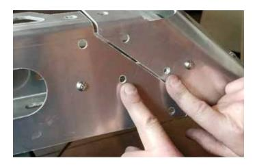
Attach front fascia piece shown bottom left photo along with a single spacer piece for each hole.
