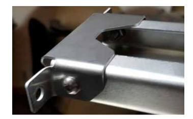
Flip roof rack on its back and attach load bars into desired locations as shown in photo. Using provided nuts and bolts, you may begin tightening down each load bar with two bolts/nuts for each side of load bars as shown.
