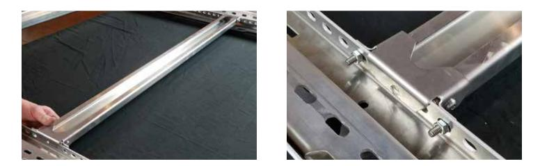
Flip over roof rack after all load bars are tightened down with tools and begin tightening all other rack bolts to prepare to mount onto vehicle.
