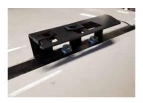
Once all mounts are put into place and tightened down, carefully place the roof rack onto the roof with a friend to line up with the mount brackets. Begin placing the provided bolts and washers into each hole and tighten down.
