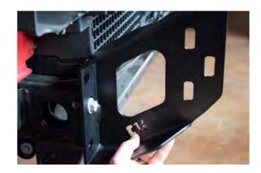
Slide in single nut retainer bracket into large hole in the back and tighten with bolt/washer as shown.
