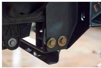
Slide provided spacer between frame brackets and secure with provided bolt, nut and washer.
