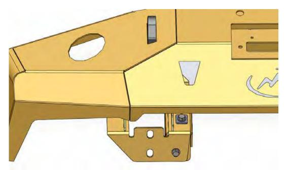
The two open holes shown in photo above are used if you want to reattach your recovery hooks. If not, you will need to screw back in the original bolts that attached the stock hooks.
