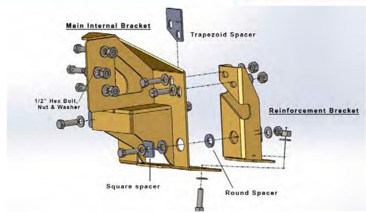
Using the 1/2" bolts provided, piece together around frame with provided internal brackets as shown in renderings above and below. Make sure to use provided square/round spacers as shown in photo above to fill in gaps between frame and brackets.
