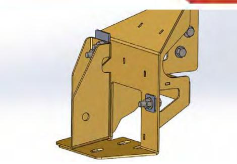
Use provided 1/2" bolts to attach your bumper onto the reinforcement brackets.
