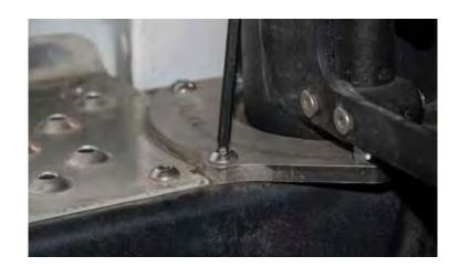
If handle needs to be adjusted, then these three bolts shown to right are the bolts you will need to adjust to do that.
