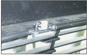
Pull the top of the bumper cover out for access to the factory grille inserts. Remove the upper factory clips from top of the grille inserts by prying them off with a small flat blade screw driver.
