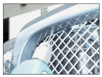
Using a 1/8" drill bit, drill through the marks made in the previous step.
