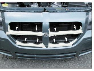
For vehicles painted other than black, use masking tape to cover the grille center bar and lower section.
