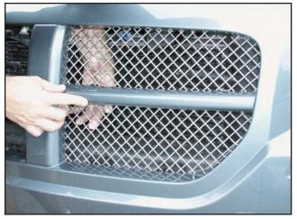
Align the left and right mesh sections behind the factory grille openings. Be careful not to scratch the paint applied to the center and lower mounting tabs.
