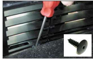
Use a phillips screw driver to remove the lower factory mounting screws and pry off the screw clips. There are two (2) large black plastic screws (see close-up) that retain the lower left and right sides of the factory grille inserts (one per insert). Remove the screws using a square drive bit (not shown).
