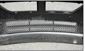
12. Lower Grille Installation: The following pictures were taken with the front end removed for photo clarity. You do not need to remove the bumper cover to install the lower grille.
