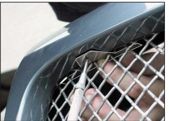
Keeping the mesh grille tight against the opening, align the upper mounting mounting brackets as shown and mark the mounting hole location onto the bumper cover.
