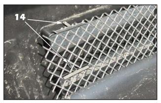
14. Align and install the lower mesh mounting brackets using the same procedure outlined for the upper mesh sections. Two brackets will be used on each side (upper and lower positions as shown), with one bracket used at the lower center. Once the brackets are installed, reinstall the lower air deflec-
