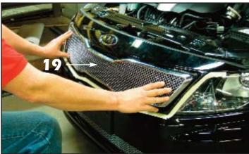
Reinstall the assembled grille back onto the bumper cover by reversing steps 12 through 16, then remove the protective masking tape.
