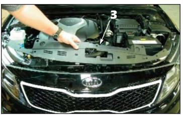
3. Lift up on the rear edge of the radiator support panel and pull it back to release the front edge from the bumper cover.
