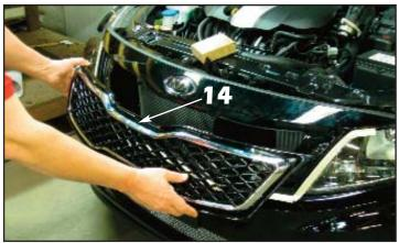
14. Carefully pull the grille straight out to release it from the bumper cover. *Use masking tape to cover the factory chrome moulding* before you remove it in the following steps. This will prevent the chrome from being scratched during the mesh installation.
