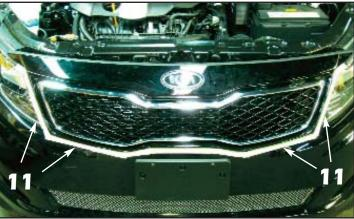
11. Apply masking tape to the bumper cover underneath and around the sides of the factory grille.
