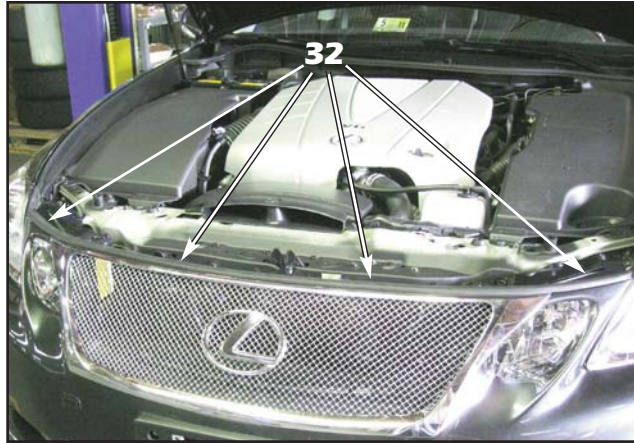
32. Reinstall the factory weatherstrip across the top of the grille assembly and bumper cover.
