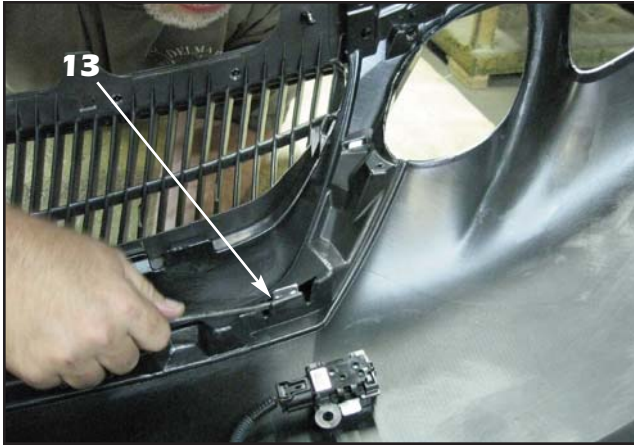
13. Use a flat blade screwdriver to unclip the lower mounting tabs and remove the factory grille insert from the bumper cover.
