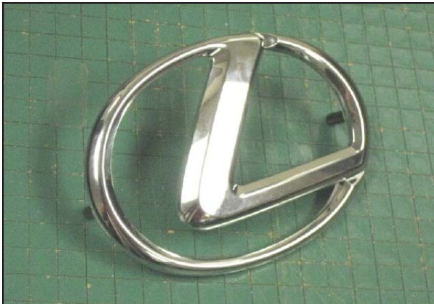
16. Peel off the double faced tape backing , make sure the alignment studs pass through the holes in the emblem mounting plate and press the emblem firmly in place to set the tape.
