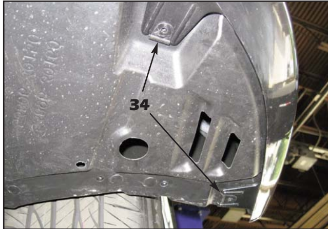
34. Make sure that the factory bumper cover tabs fit into the lower belly pan clips before you install the 10mm hex screws and plastic push fasteners.
