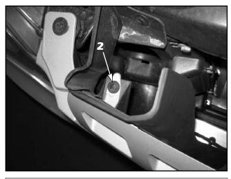
2. Remove the side push pins retaining the top sides of the factory grille.
