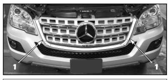
1. **IMPORTANT**: Apply masking tape to all painted surfaces of the front bumper cover around the grille opening to protect the paint from damage.
