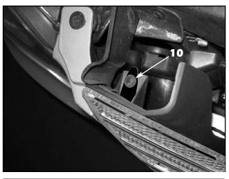
10. Reinstall the factory push pins removed in Step 2.
