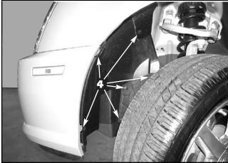
4. From underneath the vehicle: E&G recommends either lifting the car with a lift, or raising the vehicle and installing jack stands before proceding. Remove the two push pins located in the front wheel openings (each side) and four push pins located inside the wheel well.
