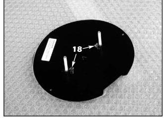
18. Once the emblems are installed, use a disc grinder to remove the alignment pins on the emblems prior to installation on the mesh grille.
