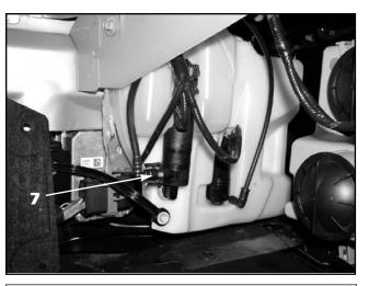
7. Disconnect and plug the high pressure headlamp washer line from the pump (C). A 1/4" I.D. rubber plug works best (not supplied). If a plug is not available, allow the fluid to drain into a clean container and refill the resevoir once the line is reconnected.
