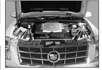
3. Remove the push pins from each side (where shown).
