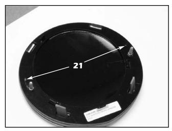
21. Install the factory wreath and crest onto the supplied emblem mounting plate, making sure that the crest alignment pins fit through the holes in the mounting plate (where shown).
