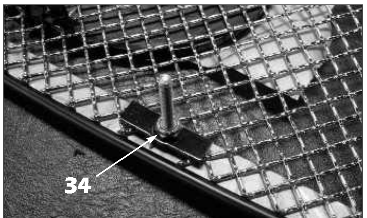
34. Install the supplied black rectangular mesh retainers across the bottom of the mesh grille using the supplied #8-32 ESNA half nuts and completely tighten.
