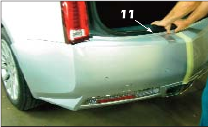
11. Pull the bumper cover free from the back of the vehicle.
