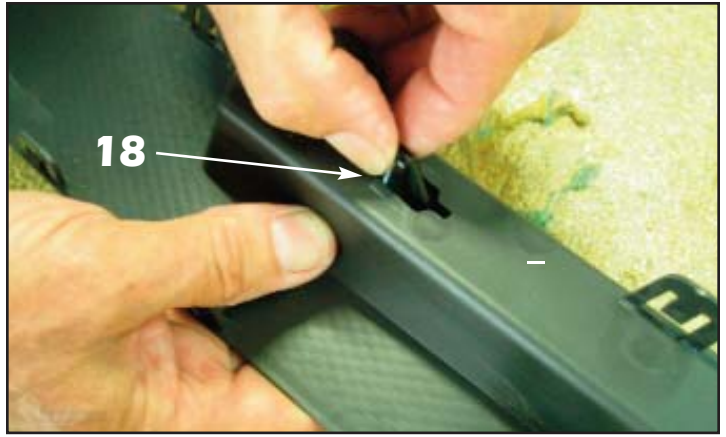
18. Squeeze the mounting clip and push the reflectors out of the gray plastic sections.
