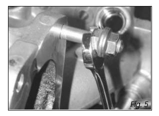
9. Connect the Fuel Filter to the fuel rail and reconnect the fuel return line. Re-fill the coolant to the factory specified level.
