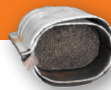
Plugged Brick Incomplete combustion by-products have plugged the holes.
