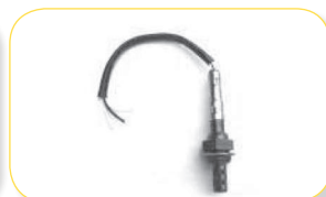
11014 Universal 3-wire 3-wire w/ 6.0 OHM heater 22mm (7/8") hex nut 18mm x 1.5 SP thread
