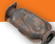
Road Damage Impact under the vehicle crushed the converter.
