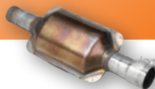
Burned Converter Exhaust temperature too hot.
