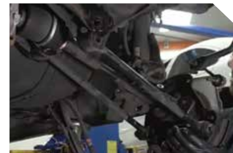
Step 4 Disconnect the strut mount at the knuckle and remove the axle assembly as a unit.
