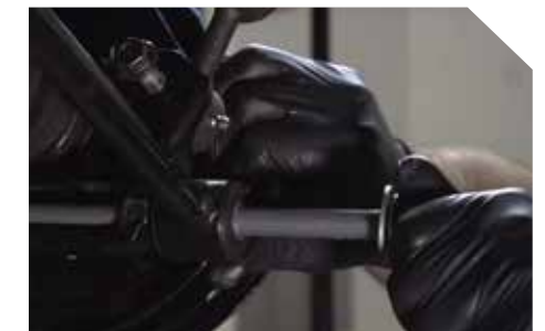
Step 6 Install new lateral link bushings, install the new loaded knuckle, and reassemble using the new through-bolt.
