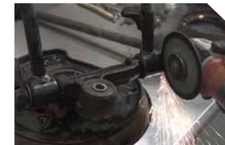
Step 5 Cut the nut off the through-bolt and remove the old bushings.
