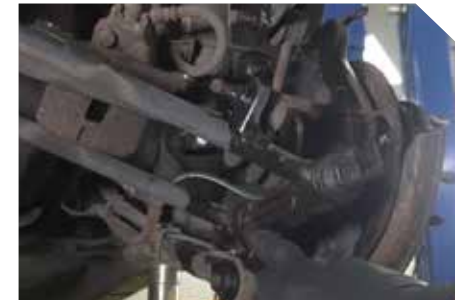
Step 1 Use penetrating solvent to soak all hardware.
