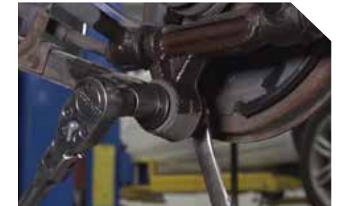
Step 3 Disconnect the trailing arm, brake hardware and sway bar from suspension knuckle.
