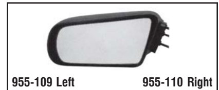
955-109 Left 955-110 Right GM 1994-88 Cavalier, Sunbird (Exc. SE, GT models). Manual Cable Controlled Color: Black
