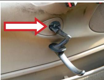
**STEP 10:** Remove the upper interior door trim retaining screw. The screw is located just above the interior door mechanism. The screw is somewhat obscure. Failure to remove this screw will not allow you to remove the door trim panel.
