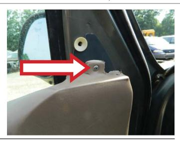
**STEP 6:** Using a small flat-blade screwdriver, place the screw driver in one of the recessed grooves in the door trim panel marker light assembly.
