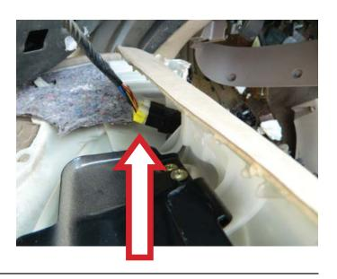
**STEP 13:** Remove the door marker light socket from the door trim panel.
