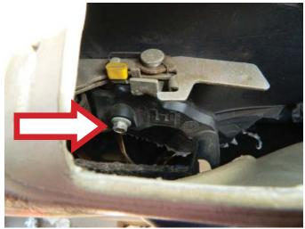
**STEP 19:** Attach the master power switch wiring onto the switch assembly.
