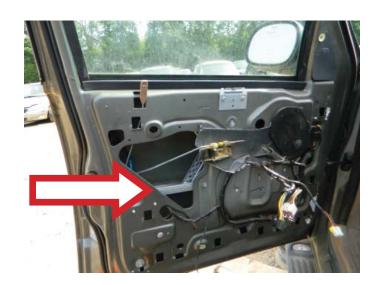
**STEP 2:** Loosely mount the window regulator assembly.
