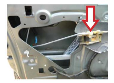
**STEP 8:** If vehicle was equipped, re-install water vapor barrier.
