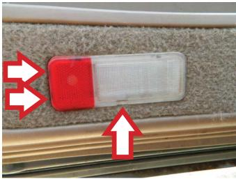
**STEP 7:** Remove the door trim panel marker light assembly retainer screw.
