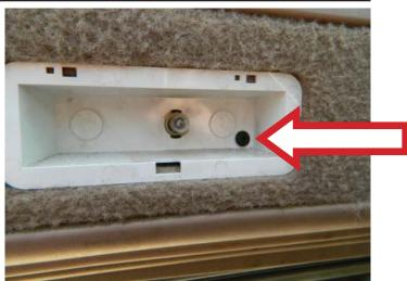
**STEP 16:** Install the door marker light assembly.
