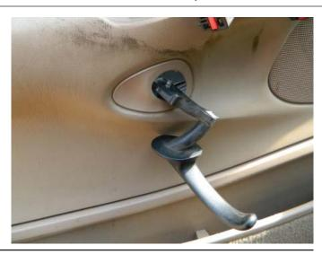
**STEP 18:** Attach the door handle retaining screw.
