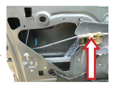
**STEP 20:** Remove the window regulator assembly through the access hole.
