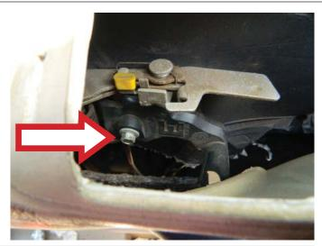
**STEP 9:** Remove the door handle assembly through the door trim panel opening.
