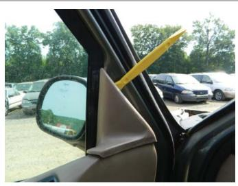
**STEP 3a:** Using a plastic trim panel removal tool, place the tool between the interior door trim panel and the rear view mirror bezel, and pry in an upward motion.
