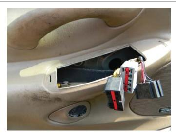
**STEP 11:** Align the door trim panel with its corresponding retainer holes.
