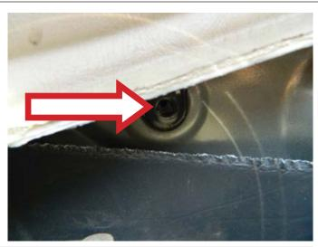
**STEP 15:** Install the door marker light assembly retaining screw.
