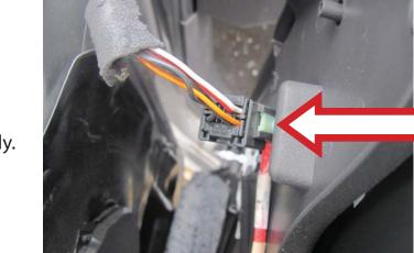
**STEP 3a:** Disconnect the power mirror connector from the door harness assembly.
