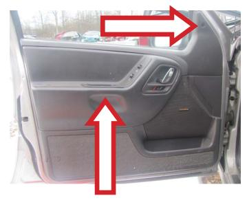
**STEP 1:** Remove the interior door trim panel attached by two (2) T-25 Torx head screws.
