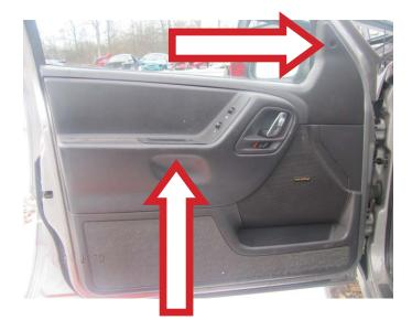
**STEP 11:** Attach the T-25 Torx screws to the interior door trim panel.
