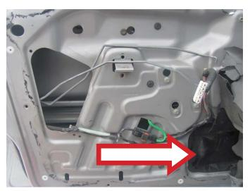
**STEP 2:** Loosely mount the window regulator into the door.
