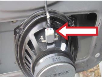
**STEP 6b:** Disconnect the door speaker connector from the door speaker.
