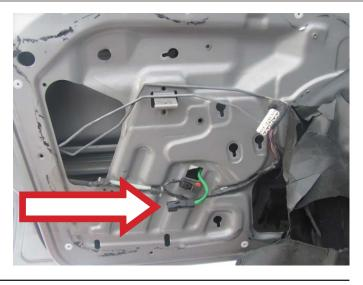
**STEP 3a:** Attach the window glass to the window regulator assembly. Take note that you may need to temporarily connect the master switch assembly to the door to operate the window regulator assembly to attach it to the window glass. **NOTE:** DO NOT OVERTIGHTEN THE ATTACHING HARDWARE TO THE GLASS. YOU WILL BREAK THE GLASS IF YOU OVERTIGHTEN YOUR BOLTS.
