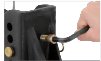
Built-in anti-rattle helps promote quiet towing (select models)
