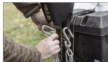
Integrated hanger bracket keeps safety chains out of the way when not in use
