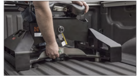
Step 3 - Secure levers with attached safety pins and you're ready to hitch up your trailer
