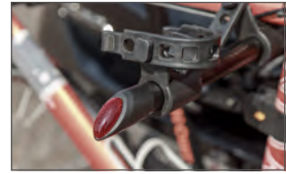
Built-in reflectors provide added visibility for safety
