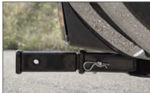
Moves coupling point farther from the vehicle to avoid obstructions
