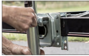
Heavy-duty pull-pin locks jack securely in place
