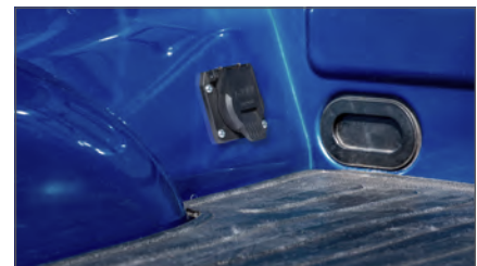
10' routes socket closer to truck cab
