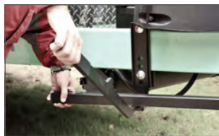
Adjustable brackets provide fixed support unlike chain models
