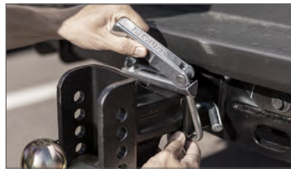
No-tool installation and easy-to-adjust clamp lever (clamp-style)
