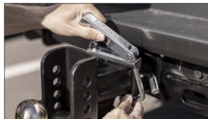
No-tool installation and easy-to-adjust clamp lever (clamp-style)
