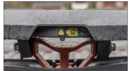
Three-position coupling indicator clearly shows coupling status
