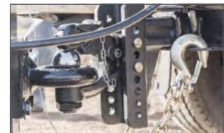
Helps resist total vehicle-trailer separation during a disconnect
