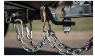
Provides intermediate hangers to keep safety chains off the ground
