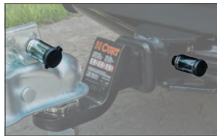
Watertight dust caps prevent internal corrosion
