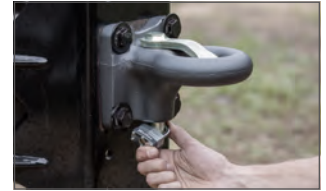
Drop-in pin accepts lock to deter theft (turns 90° while coupled)
