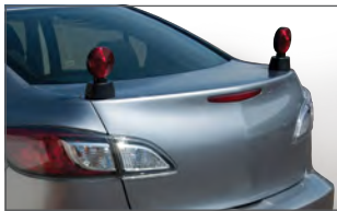
Easily adds tow lights to a vehicle being dinghy towed
