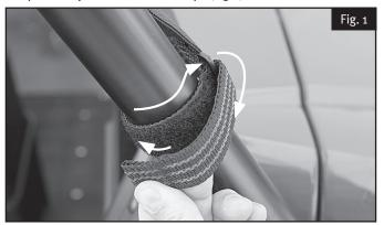
**2.** Adjust the top straps and then the bottom straps to position your Windshield in the center of the roll cage uprights (Fig. 2). When it is centered and level tighten all the straps.
