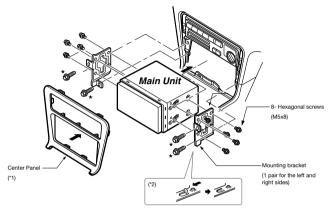
\*1. Some panel openings are too small for the unit depending on the vehicle type and model. In such a case, trim the upper and lower sides of the panel frame by about 0.5 to 1.5 mm so the unit can be inserted smoothly.
