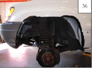
Completed cut-out with caulking applied.
