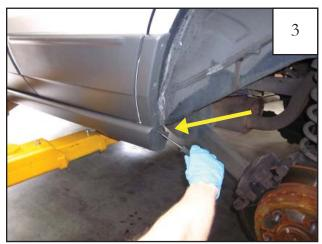
(Note: For models with Rocker Panels installed) Using a #2 Phillips Screwcriver, remove screw from rocker panel in rear wheel well.
