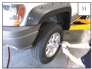
Re-install tire using an impact wrench.
