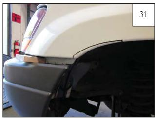
Use a small wood block to prop the bumper away from the fender in preperation for sheet metal trimming.
