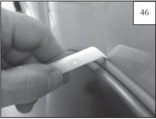
Using supplied Edge Trim Tool (ET1-0002), seat edge trim against vehicle by hooking curved end under edge trim at one end of flare. Next, slide around outer edge of flare to the other end. You should repeat this process once screws are tightened.
