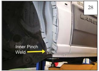
Mark the inner pinch weld with 5 lines appoximately 2 inches apart starting from the bottom.
