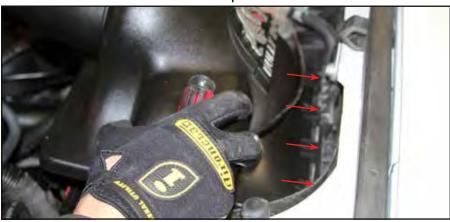
2. Secure RFI lid to the stock box by closing the latches on the box.
