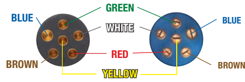
TRAILER END As viewed from core back side where wires are attached with screws.
