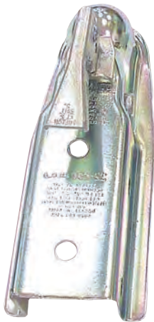
Fulton coupler after 336 hours salt spray testing.
