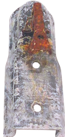
Competitor's coupler after 336 hours salt spray testing.
