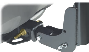
Tighten nut on J-Pin shaft, compressing ball mount or hitch-mounted accessory against receiver tube
