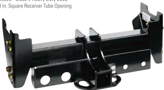
38023 - Class V Heavy Duty 3000 3 in. Square Receiver Tube Opening
