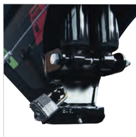
Lockable BULLDOG® coupler for added security
