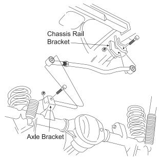
HINT: The factory rear trackbar bracket on axle utilizes a "pocket" design that requires the Adjustable Trackbar be removed from the chassis bracket before Axle End (A) can be inserted. This may not be necessary if an aftermarket extension bracket has been installed on the factory axle bracket.
