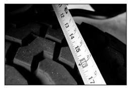
**HINT**: For example, measure from the edge of a tire tread lug to the outboard side of chassis, then repeat the measurement on other side of vehicle using exact same points.
