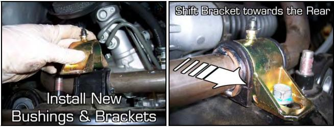
*Use bracket with the 90° grease fitting for the front. Fitting points out board. Straight fitting is shown in pictures for prototyping.*
