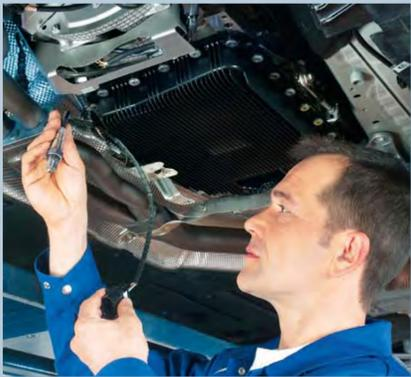
Oxygen sensors are important engine components indispensable for reliable engine function and correct emission values. But the perfect functioning of oxygen sensors can be jeopardized by many factors:
