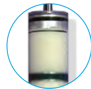
Non-pressurized shock, foaming
