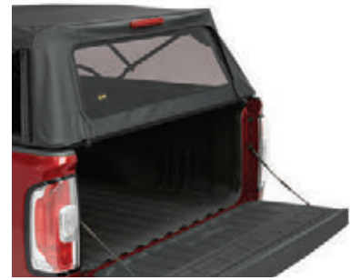
Tailgate opens with window installed
