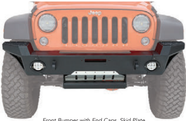
Front Bumper with End Caps, Skid Plate, and Approach/Departure Roller
