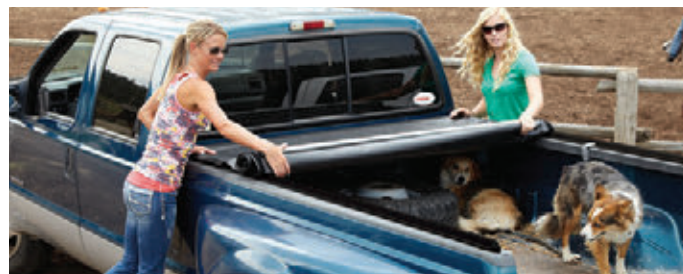
Roll-style tonneau, attaches with hook-and-loop fastener, mounts on top of bed rails
