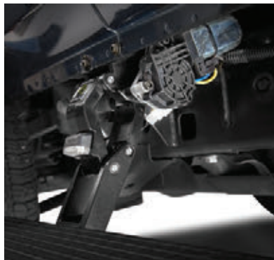
Powerboard Motor Detail
