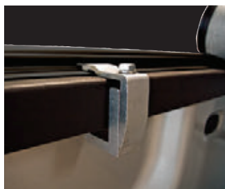
No-drill installation clamps secure frame rail assembly to bed
