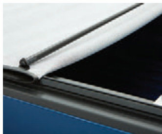
Fully-integrated bow system for smoother profile and easier install
