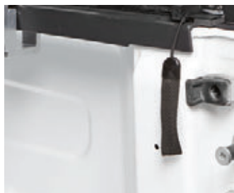
Pull tabs at both rear corners for convenient operation
