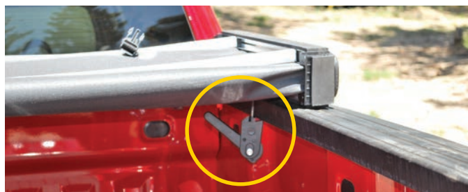
Heavy-duty adjustable clamps secure tonneau to truck bed
