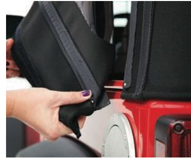
Black Twill has 40 mil, DOT-approved vinyl side and rear windows that attach to existing Belt-Rail system
