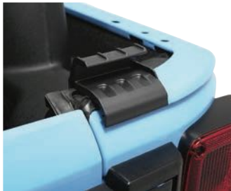
Use of tailgate bar and clips allows hassle-free opening of tailgate
