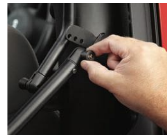
Adjustable bow system helps keep fabric taut and includes Bestop® quick-release bow knuckles
