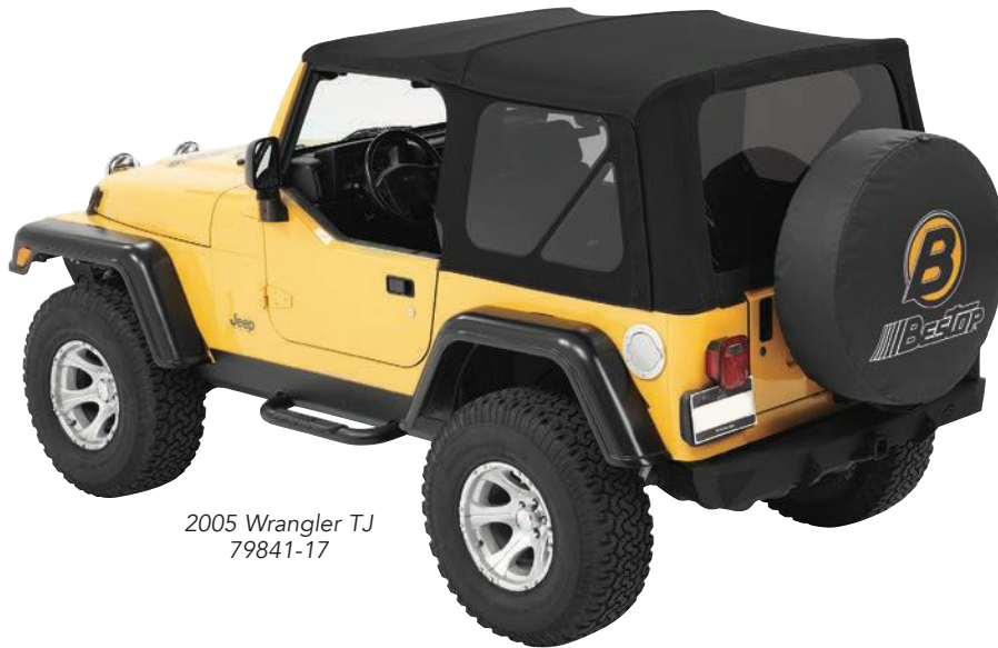
Black Twill has 40 mil, DOT-approved vinyl side and rear windows that attach to existing Belt-Rail system
