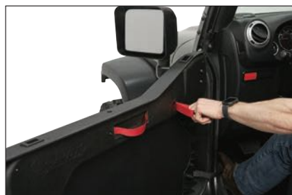
Remote latch release and OEM-quality check strap
