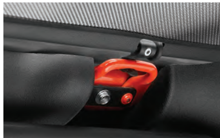
Sunshade securely latches to footman loops
