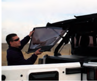
Combination of zippers and zipperless channels makes window install and removal seamless
