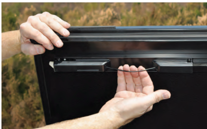
ACCESS RELEASE CABLES ON EITHER SIDE
