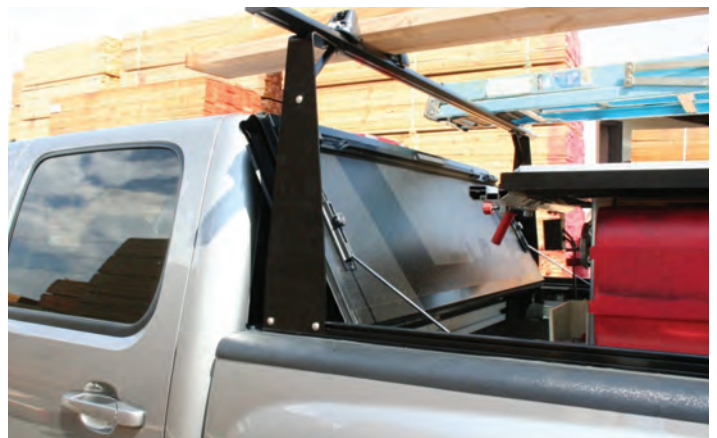
COVER FLIPS UP TO HAUL LARGE EQUIPMENT
