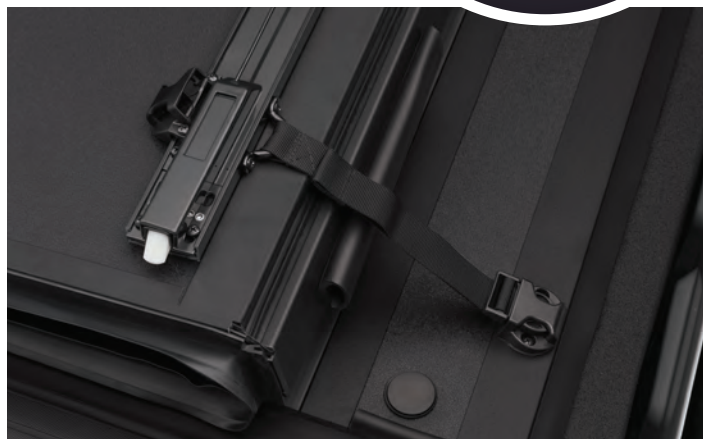
BUCKLE SYSTEM SECURES COVER IN FOLDED POSITION
