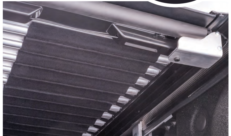
UNDERSIDE REVEALS STRONG ALUMINUM SLATS
