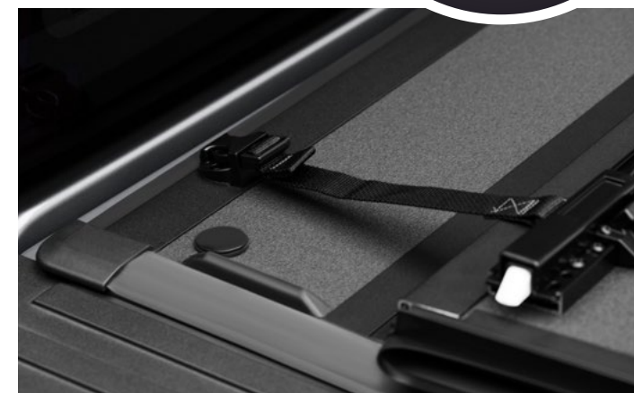
BUCKLE SYSTEM SECURES COVER IN FOLDED POSITION
