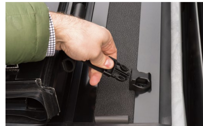
BUCKLES SECURE COVER IN FOLDED POSITION
