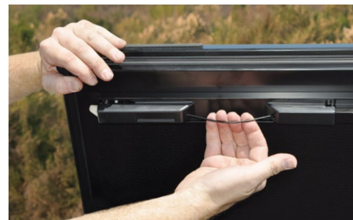
ACCESS RELEASE CABLES ON EITHER SIDE
