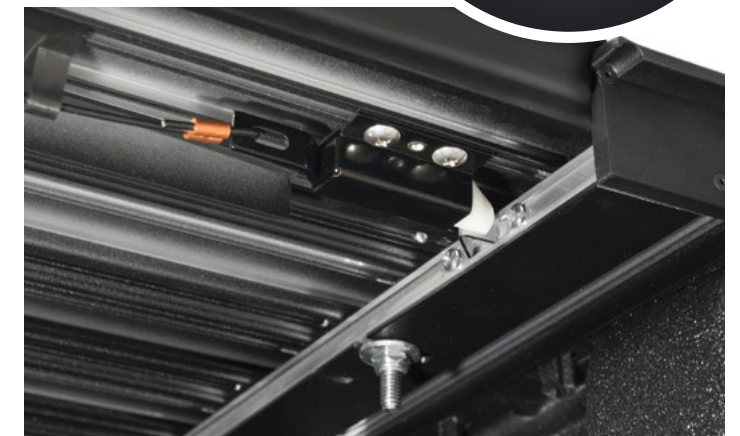
RELEASE CABLE OPENS COVER FROM DRIVER OR PASSENGER SIDE
