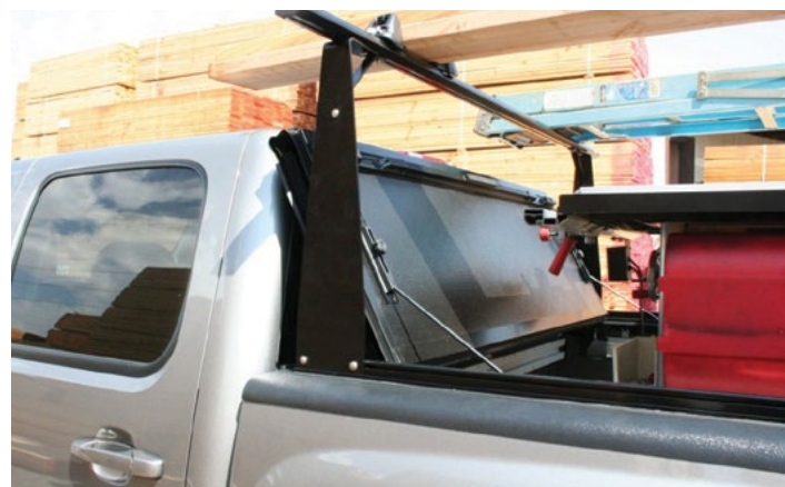
COVER FLIPS UP TO HAUL LARGE EQUIPMENT
