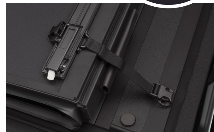
BUCKLE SYSTEM SECURES COVER IN FOLDED POSITION
