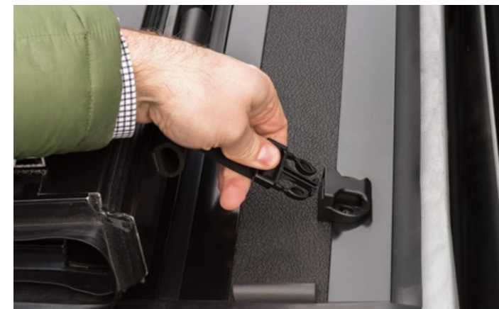
BUCKLES SECURE COVER IN FOLDED POSITION
