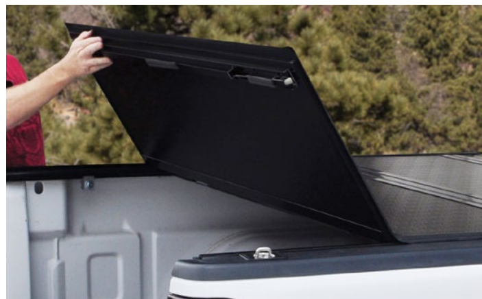
FOLDS OPEN WITH SIMPLE RELEASE CABLES
