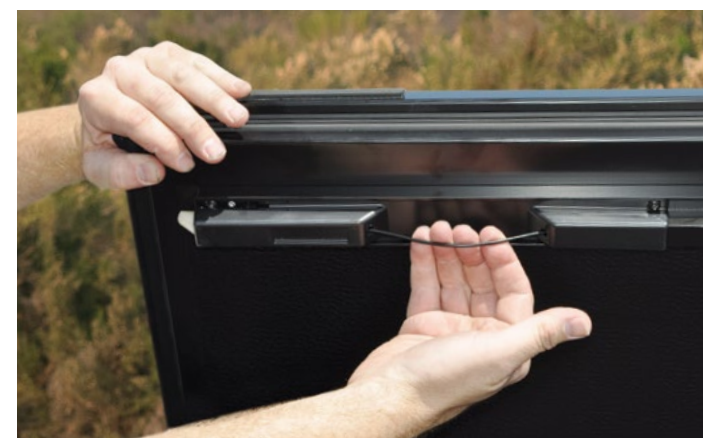
ACCESS RELEASE CABLES ON EITHER SIDE
