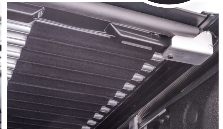
UNDERSIDE REVEALS STRONG ALUMINUM SLATS
