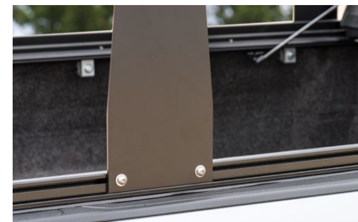
RACK UPRIGHTS EASILY SLIDE ALONG CARGO RAILS
