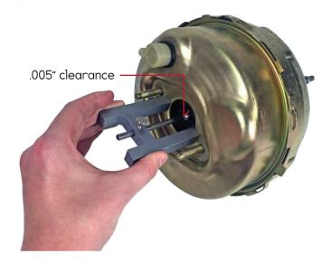
Tool Positioned On Booster
