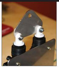
Take the triangle mount and the 1/2'' nut & bolt and secure it to the actuators's arm (the white fixture).
