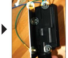
Align the actuator mount screw holes with the actuator's. Secure the actuator to the mount using the 1/4" screws. \*Special Note - you might want to pre thread the actuator screw holes before attaching it to the mount for easier installation.
