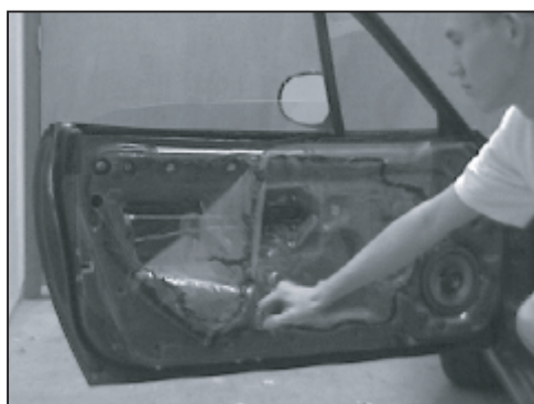
5. Carefully remove the clear PVC protective sheet from the door.
