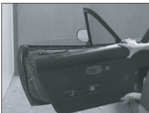
4. Remove the door's interior panel by inserting a screw driver between the door, and door panel. Once inserted pry off the door panel by pushing or pulling on the screwdriver.
