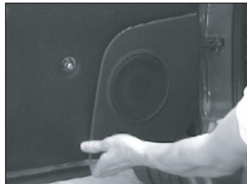
3. Remove the door's speaker panel by inserting a screw driver between the door, and speaker panel. Once inserted pry off the speaker panel.
