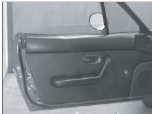
2. Remove all the handles, fittings, and arm rests from the door.
