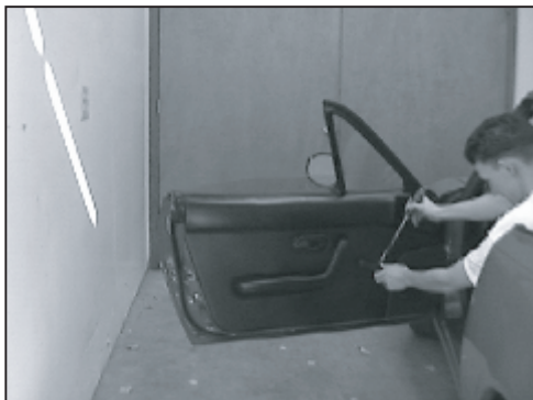
1. Using a flat screwdriver remove the "c" clip from the window crank.
