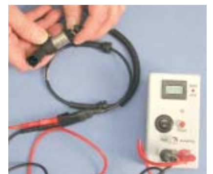
Sensor tester used on dismantled active sensor
