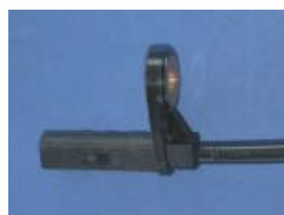
Active wheel sensor for axial pick-up
