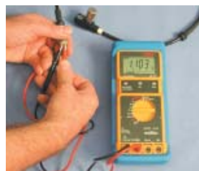
Testing of passive sensor
