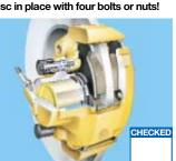
• Free running of caliper, sliding elements and piston checked?
