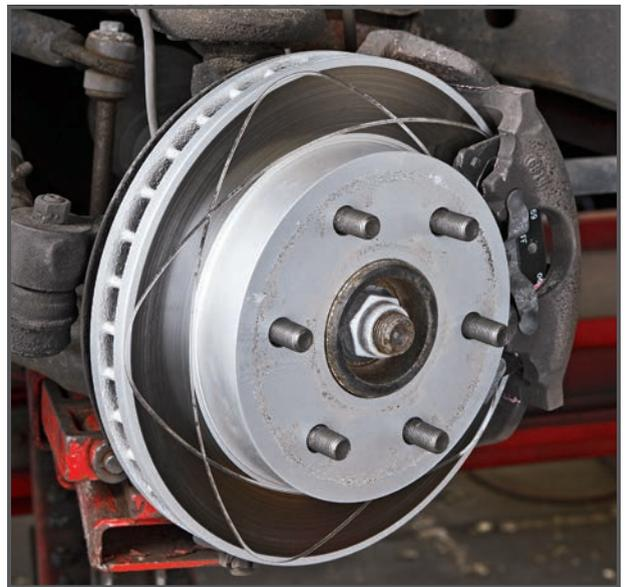
Although this vehicle has been on the road for a while, the MetaCote finish on the ATE PremiumOne rotor has prevented any new rust from developing on the rotor.
