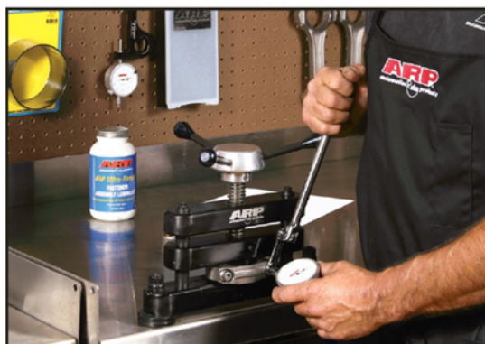
A rod bolt stretch gauge is one of the most important tools a serious engine builder can own. It's valuable in properly setting up a rod for resizing, obtaining the proper torque load when installed in the engine, and monitoring the condition of the bolt while in use.
