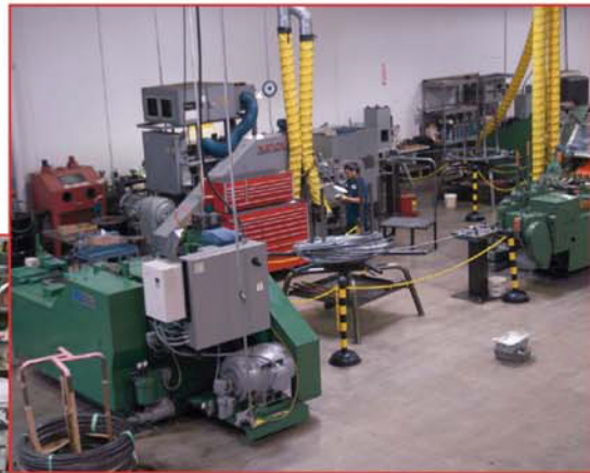
Powerful cold-forging equipment is used to make ARP's hex and 12-point nuts. Multi-stage dies are employed to precision-form the finished “blanks.”
