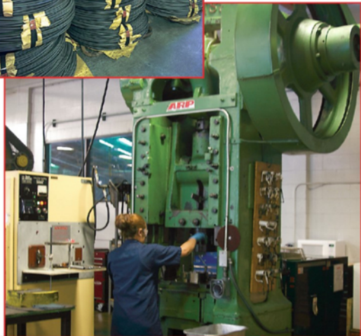
Material comes from the mill in large coils...which subsequently will be fed into cold-headers and formed into bolts.
