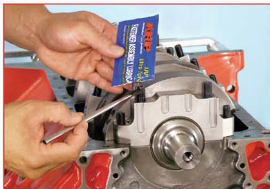
4. Install main caps, checking for binding and misalignment. Lubricate threads, nuts and washers with ARP Ultra-Torque fastener assembly lubricant before installation. Have the block align honed.
