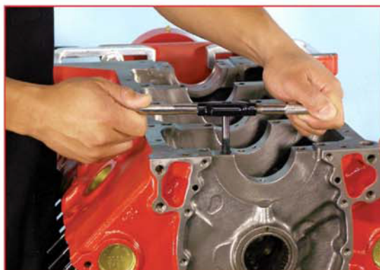
1. Clean and chase appropriate threads in block to ensure proper thread engagement and accurate torque readings.
