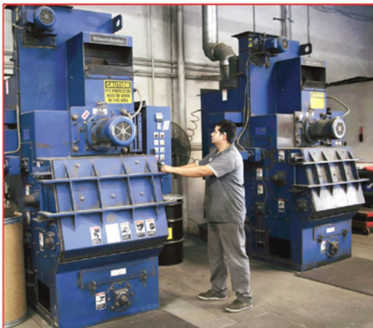
Fasteners are shot-peened after heat-treatment to improve overall external integrity.
