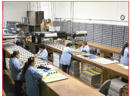
Components for each kit are placed on the appropriate display cards, sealed and labeled. Through-put has been significantly increased.
