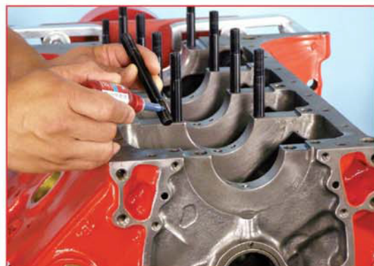
3. Screw studs into block, finger tight ONLY. For permanent installation, apply Loctite (or similar adhesive) sparingly to threads. Be sure and install the caps promptly before the cement sets to prevent misalignment of studs in block.
