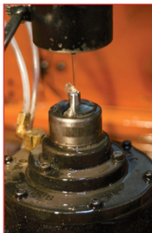
State-of-the-art EDM technology is used to perform special operations, such as hex-broaching the nose of a unique short-run fastener.
