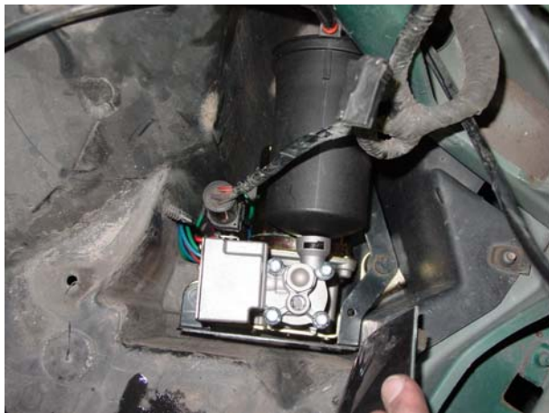
15. Install new compressor on vehicle. ↑ (Reverse steps 3-14)
