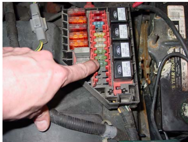
17. Replace the 30 amp fuse for the air suspension motor.
