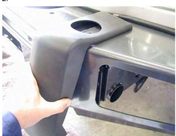
Insert the side buffers through the holes and fix using the M6 flange nuts. (Do not over tighten)
