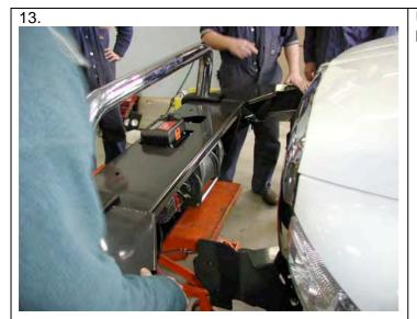
Using two people, three if winch fitted, position the bar assembly on the vehicle mounts.
