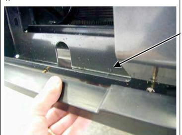
Position the lower buffer on the winch bumper and assemble using the M6 flange nuts. (do not over tighten)
