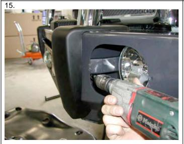
The bar must be pin bolted to the mount brackets. Using a drill and 10mm drill bit, drill through the upper and lower Ø10mm holes located in the mount brackets.
