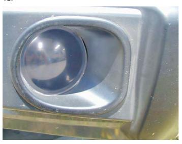
Glue the light surrounds to the bar using a silicone based rubber adhesive. Run the bead along the cavity on the rear side of the part. Position the surround to align the inside edge with the buffer and concentric to the light.
