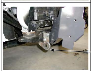
Fasten the mount brackets and tow hooks to the end of the chassis rails using M10 bolts, M10 flat washers and M10 spring washers.
