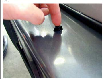
There are two Ø16 holes located on the top face of the bar. If no CB aerials are fitted the holes can be covered with the plastic plugs provided in the fitting kit
