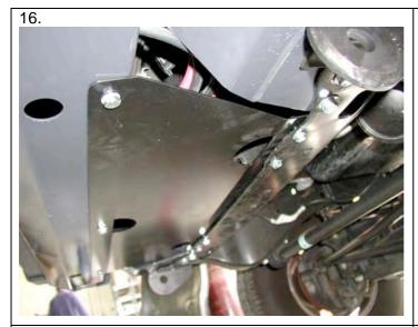
Bolt the air deflector to the underside of the bar and chassis cross member using M8 bolts, M8 flat washers and M8 spring washers.
