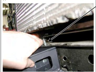
Fasten the top hole using M10 bolts, M10 flat washers and M10 spring washer.
