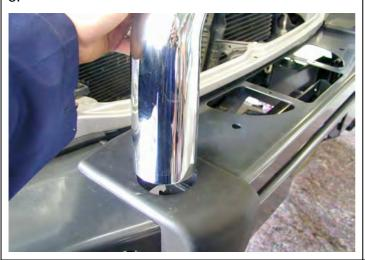
Push the top chrome tube through the hole in the buffer and fasten using the M12 x 40mm bolts, washers and spring washers.
