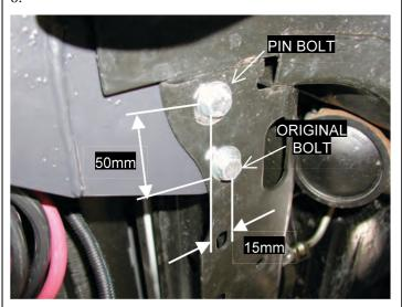
The mounts need to be pin bolted to the vehicle chassis.
