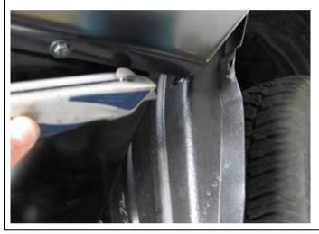
94. Carefully trim off the bottom of the guard liner flush with the wing under panel
