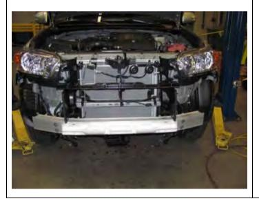
29. Remove reinforcing beam foam pad, then remove the beam, *refer next step*.
