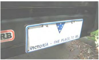
87. The licence plate can now be attached to the bull bar. Insert the two plastic square plugs supplied into the two square holes in the face of the bull bar (note slot allows for adjustable number plate hole pitch, ensure grommet flanges fit over the narrow width of the slot to engage correctly).
