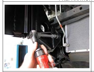
46. Fit impact absorbers to chassis ends using fine thread M10 x 1.25P x 30 bolt and washer sets supplied, note that the brackets are handed, slide them towards the centre of the vehicle on the adjustment slots do not do up tight
