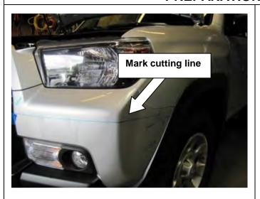
4. Mark a straight, horizontal line joining the marked cutting points on each end of the bumper
