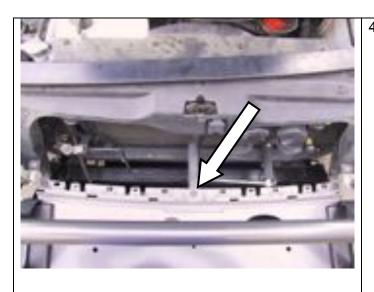
11. Take cut out trim from OE bumper (Step 4) and tuck leading edge of plastic trim under back edge of bumper and use OE retaining clips in the OE holes to hold bumper piece into place
