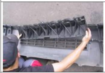
1. Undo bumper light electrical connections and then remove front bumper cover from vehicle
