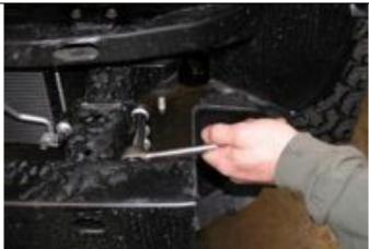
7. Remove front bumper reinforcing bar. NOTE: Retain the 8 x flange nuts removed for fitment of the bull bar chassis mount.
