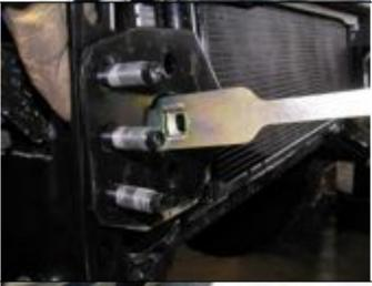
13. Insert the captive nut assembly through the front of the chassis and line it up with the hole at the end of the mount brace. Fix in place with the M12 x 1.75 x 40mm bolt, M12 flat and spring washers. Break off the end of the captive nut plate. Do not tighten yet.
