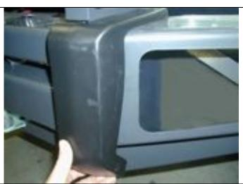
31. Fit the buffers to either side of the bull bar using 6 x M6 flange nuts. Do not over tighten.
