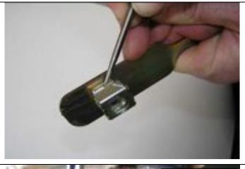
11. Fit an M12 cage nut to each of the captive nut plates 3193741.
