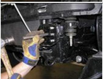
Check that the nut body is completely removed, if it is not cleared, using a cold chisel and hammer chisel the remainder off.
