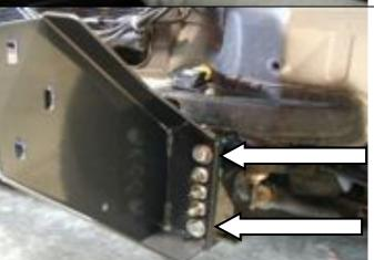
17. Fix the chassis mount bracket to the chassis mount brace using M12 x 40mm bolts, M12 spring and flat washers, the 8mm spacers and M12 x 1.75 nuts. Tighten bolts
