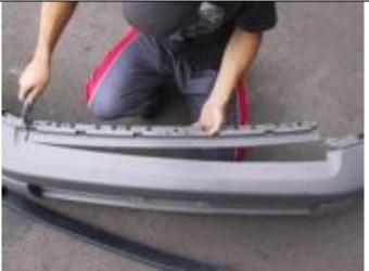
4. Remove trim and then cut out plastic panel along marked line from OE bumper facia, set this piece aside for fitting later.
