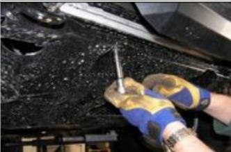
8. Remove front fasteners only from stone tray. Retain fasteners for reuse.
