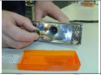
38. Replace 21W light bulbs for indicator (yellow reflector side) in supplied indicator/run lamp assemblies with 10W bulbs from fitting kit.
