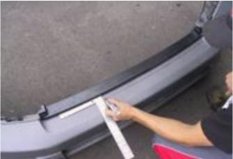
3. With trim piece fitted to OE bumper cover as shown, mark out and draw a line 25mm (1") from the leading edge of the lower grille trim approx. 864mm (34") long
