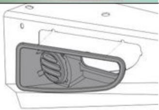
39. Assemble and install combination light surrounds (p/n 3163015) as per instructions no. 3786421 supplied with surround kit. Note: Optional fog lamps can be installed at this point as per fitting instruction no. 3783315 supplied with fog lamp kit 6821201
