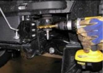
Using the 13mm drill bit and power drill, drill out the M8 captive nut located at the outboard side of the chassis as shown, on both sides of the vehicle.
