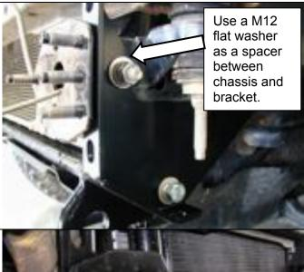
12. Fit the chassis mount braces to the vehicle using the M12 x 30mm fine pitched bolt, M12 spring and flat washers supplied in the lower hole. Use an M12 flat washer as a spacer between the brace and the chassis at the upper hole and fix with an M12 x 40mm bolt M12 spring and flat washers and M12 x 1.75 nut. Do not tighten the bolts.
