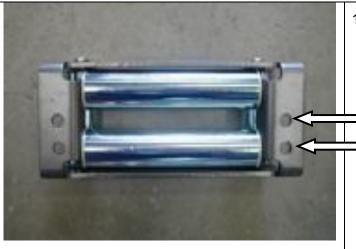
19. Using a 12mm drill bit, drill two new holes in the roller fairlead 25mm below the original holes.
