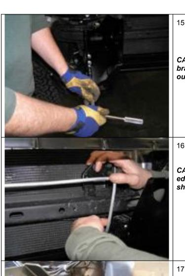
15. Fit the chassis mount bracket to the chassis using the original flange nuts removed with the bumper reinforcing bar. Centre the chassis mount bracket and tighten.
