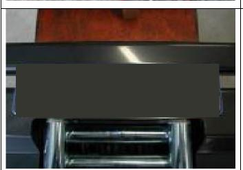
30. Insert square grommets into holes in front of bar for licence plate fixing. Place the doublesided tape along the top edge of the number plate. Using supplied black screws, attach the licence plate to the bull bar.
